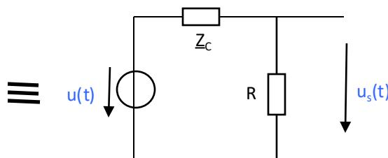
$$\frac{\underline{u}_s}{\underline{u}} = \frac{R}{R + \underline{Z}_C} = \frac{R}{R + \frac{1}{j\omega C}} = \frac{j\omega RC}{1 + j\omega RC} = \underline{H}(j\omega)$$
