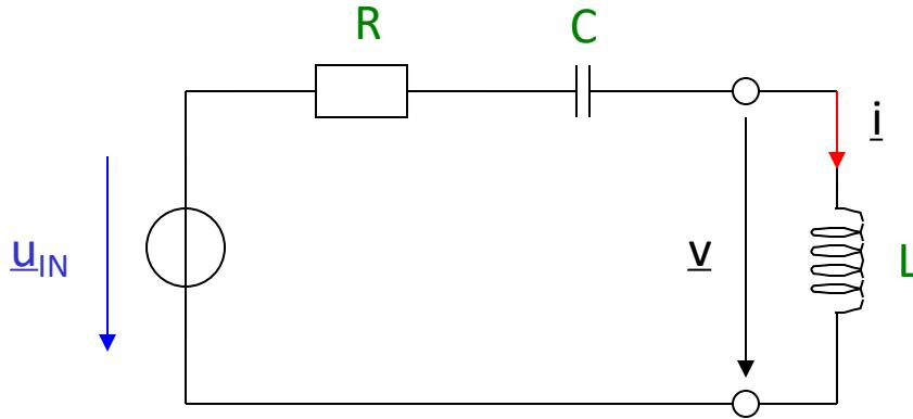
$$\underline{u}_{IN} = R\underline{i} + \frac{\underline{i}}{j\omega C} + j\omega L\underline{i}$$
